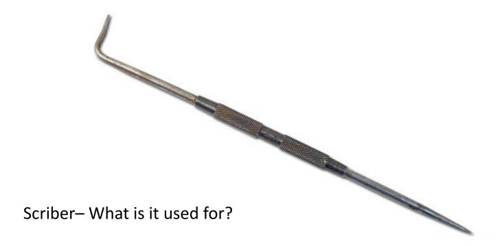
Marking out – scribing lines and features on metals.
