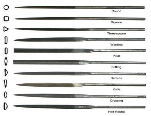
They are made from High carbon steel (HCS) which is hardened & tempered but the end "hand grip" is left soft – Why?
