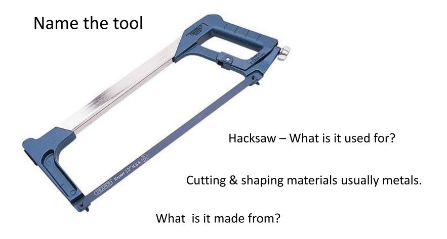
The body is made from Cast Steel. The interchangeable blade can be made from High carbon steel (HCS) which is hardened & tempered. But for the best performance (HSS) High speed steel is used.
