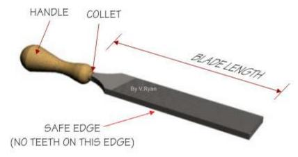
Hand files are normally held in both hands. The file is held flat against the surface it is to cut / smooth. The file is then pushed forward and it cuts on the forward stroke. It is then lifted away from the metal and returned to the starting point for the next push forward. This is called 'through filing'
