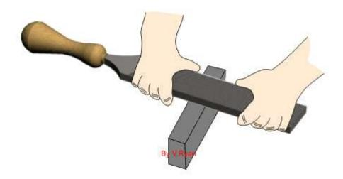
The final stage of filing / smoothing a piece of metal / plastic is to use either emery cloth or wet and dry paper. Emery cloth is used for metals whilst wet and dry paper is used for plastics. The cloth / paper is held onto the blade of the file as shown i the diagram below.
