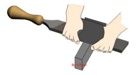
The safe edge of a file does not have teeth. This is extremely useful when filing in corners as shown in the diagram below. The safe edge is placed into the corner and because it is smooth it does not damage the surface of the metal.
