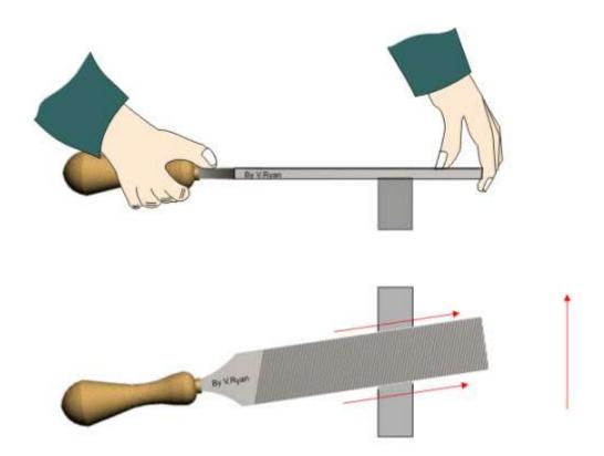
Through filing is normally the first stage in smoothing a piece of metal or plastic.
