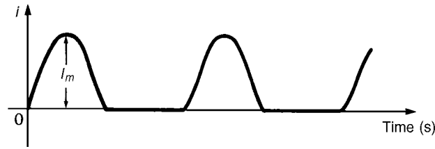
Figure 36.19 Typical current waveform containing a fairly large second harmonic
