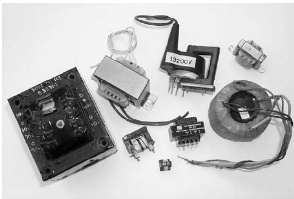
Figure 24.1: A selection of transformers with power ratings from 0.1 VA to 100 VA
