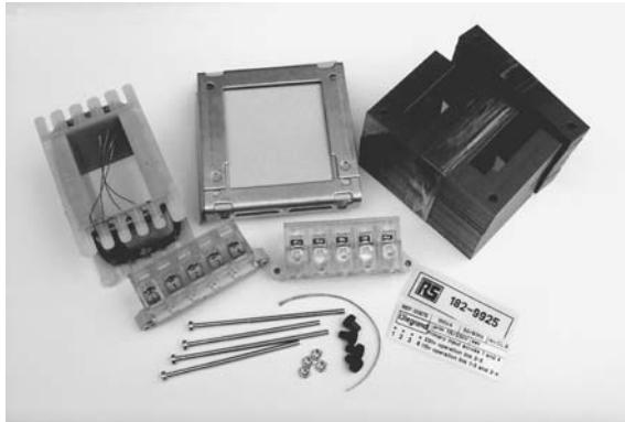
Figure 24.2: Parts of a typical iron-cored power transformer prior to assembly
