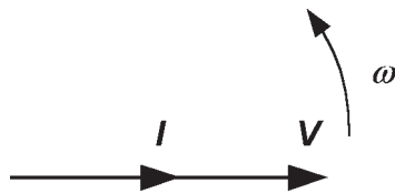
Figure 3.3.54 Phasor diagram for the circuit in Figure 3.3.53
