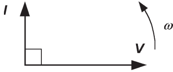
Figure 3.3.59 Phasor diagram for the circuit in Figure 3.3.58
