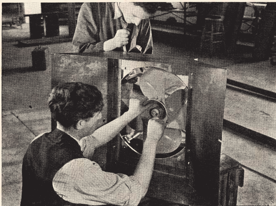
Fig. 10.—A MODERN SHEET-METAL PRODUCT Lining up position for air fan. (By courtesy of Tecalemit, Ltd.)
