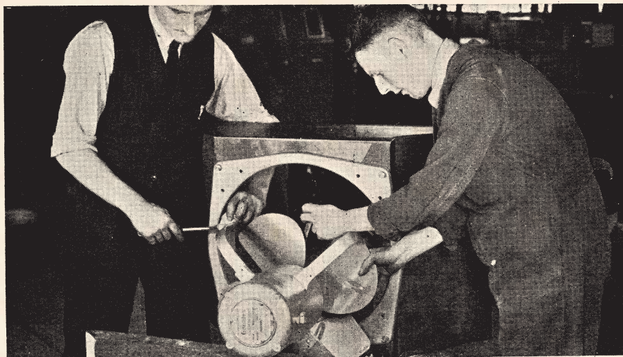
Fig. 9.—A MODERN SHEET-METAL PRODUCT Fixing an air fan to its sheet-metal case.
