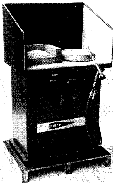
Fig. 56 A larger Alcosa brazing bench, fitted with a rotary table. The blower for the torch is set within the casing. Note the gas control cocks. (Courtesy W. Allday & Co., Ltd)
