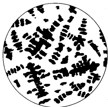
Fig. 11 A similar micrograph to Fig. 10 but for a 30% tin alloy. The dark patches are lead-rich alloy, again surrounded by the eutectic material.
