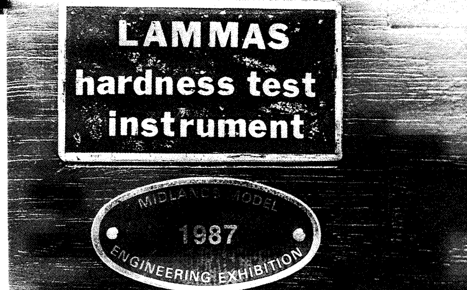
Etched brass nameplate secured to wooden base with contact adhesive.
