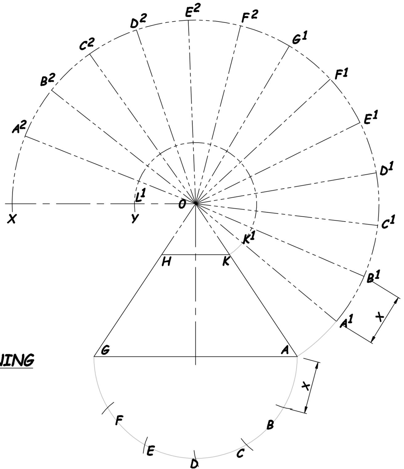
**PROCEDURE TO PRODUCE A CONE**
