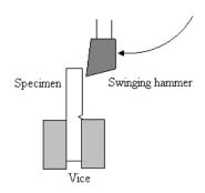
The picture shows an Izod tester for plastic specimens (The MAT20 from TQ) http://www.tq.com
