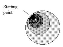
When the crack has spread enough to reduce the cross sectional area of the material to a point where it can no longer carry the load, sudden failure occurs. Often the fracture has an OYSTER SHELL appearance due to the early stages being worn smoother than the later stages.
