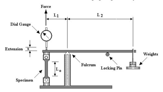
The lever is locked in place by a locking pin. A weight is added and the dial gauge is adjusted to zero. The locking pin is removed and a stop watch started at the same moment. Recordings are taken of extension and time. These are plotted to produce an extension time graph. A better machine would use electronic instruments and plot the graph automatically.
