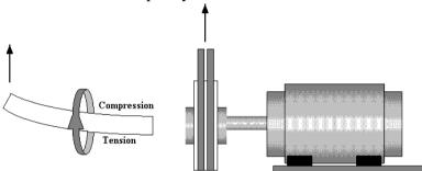
The shaft bends as shown producing tension on one side and compression on the other. As the shaft rotates, any given point on the surface experiences a direct stress that changes from tension to compression once every revolution. The alternating or fluctuating stress causes the failure. A stress - time graph is likely to be sinusoidal in a case like this.
