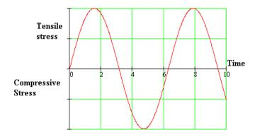
The fatigue life of a component depends on the values of the fluctuation, the mean stress level and the way the stress varies with time. This is not covered here.
