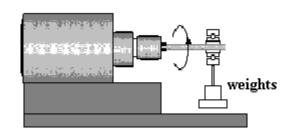
maximum stress is easily calculated. The test is repeated with different weights and hence different stress levels. It is rotated until it fails and the number of revolutions is counted. This is the number of stress cycles to failure.
