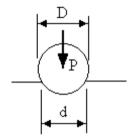
$H_{\text{B}}$  is the Brinell Hardness number, D is the diameter of the ball and d is the diameter of the indentation.
