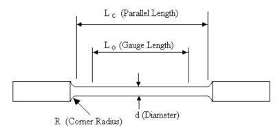
The specimens have standard cross sectional areas and so the diameters are not round numbers. The test should be conducted on approved machines. The specimen is stretched between two chucks and both the tensile force and extension are measured over a wide range until the specimen breaks.
