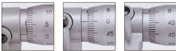
(a) From above the index line (b) Looking directly at the index line (c) From below the index line
