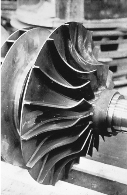
FIGURE 12.102 Three-dimensional, welded impeller. ( Dresser-Rand Company, Olean, N.Y. )
