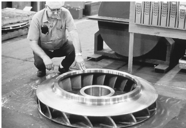
FIGURE 12.43 Three-piece welded impeller. ( Dresser-Rand Company, Olean, N.Y. )
