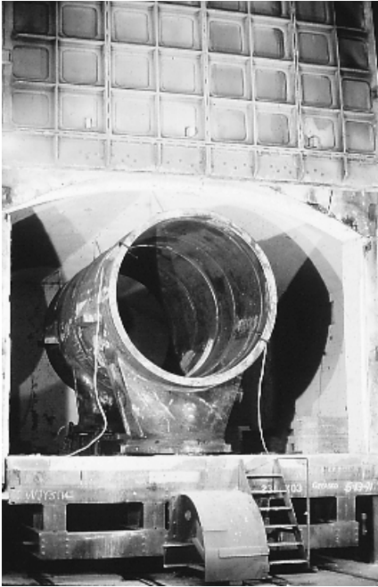
FIGURE 12.94 Heat treatment of a welded casing. (Dresser-Rand Company, Olean, N.Y.)
