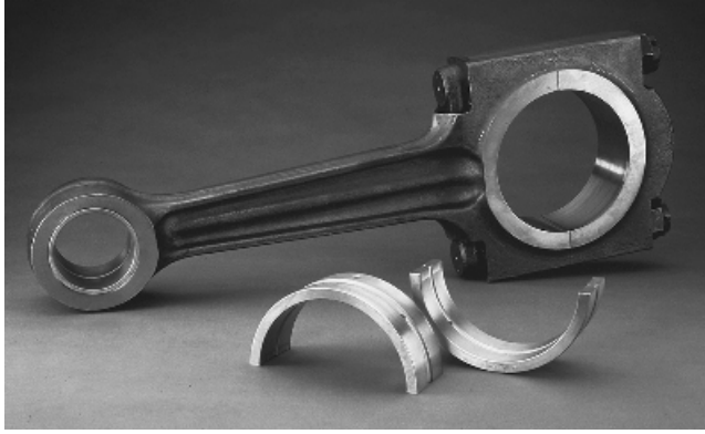
FIGURE 2.15 Typical connecting rod. ( Dresser-Rand Company, Painted Post, N.Y. )
