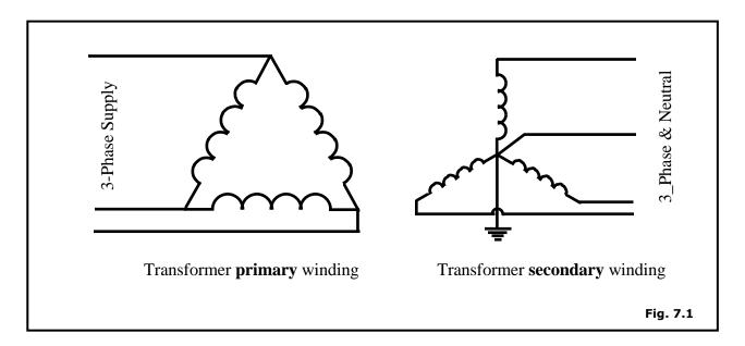
An insulation failure on the secondary side of the transformer, or on its associated system, will result in the current returning to the star point. Due to the unreliability of the earth as a conductor, (seasonal ground conditions can affect the total resistance of the earth path), protective devices are installed to continuously monitor the system and will isolate the supply in the event of a fault condition.
