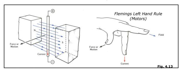
The reaction between the current and the magnetic field through which it is passing causes a mechanical sideways force on the conductor. If the conductor is free to move, it will move
