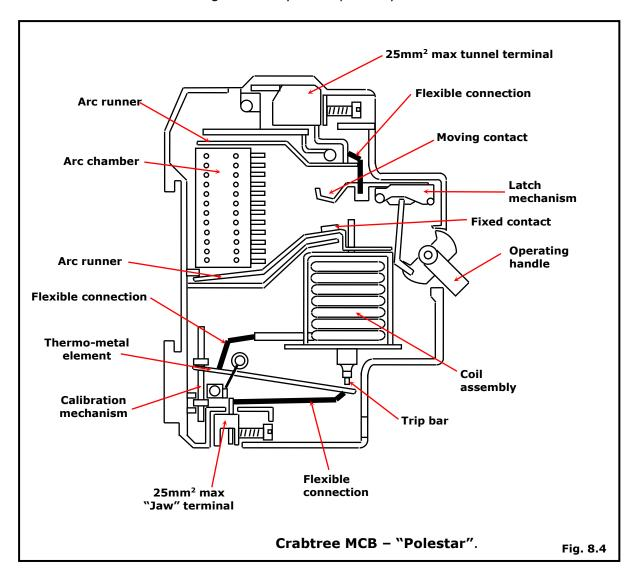
The Miniature Circuit Breaker has been designed to accommodate a variety of loads under different potential fault conditions however the correct type must be installed for a specific type of load, as described overleaf.
