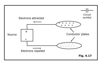
between them is equivalent to that across the source, at which point the current flow will be zero. When the source is removed the charge is released in an attempt to maintain the potential difference across it however it eventually decays to zero.
