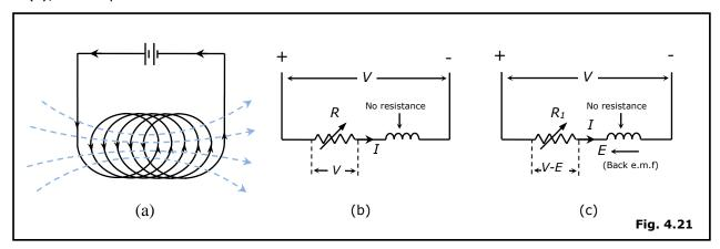
In Fig. 4.21(b), a voltage V is applied through a variable resistance R to the coil. For any given setting of R the current I through the coil (assumed to have no resistance of its own) is given by Ohm's Law hence:
