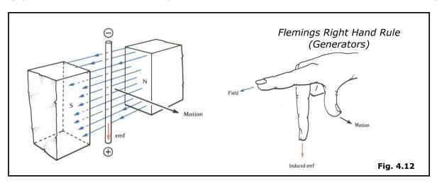
The magnitude of the voltage induced in the moving conductor entirely depends on the strength of the magnetic field and the speed of movement.
