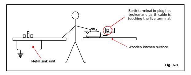
Due to the broken earth cable touching the live conductor, the metal casing of the appliance has become "live". If an individual should inadvertently touch the appliance and an earthed metal surface, as in the diagram above, then the individual will receive an electric shock.
