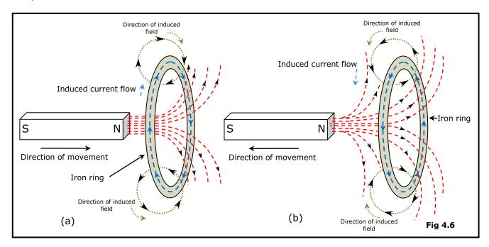
Note that the direction of the induced magnetic field within the ring is oriented so that it opposes the change in magnetic field resulting from movement of the bar-magnet.
