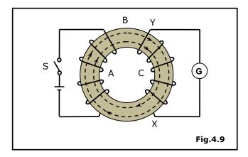
**Faraday's Law**, as it is referred, states that "the magnitude of the induced electromagnetic force (e.m.f.) is proportional to the rate at which the magnetic flux passed through the coil is varied".
