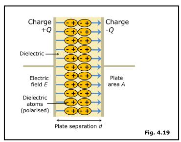
The dielectric constant is the ratio of electric flux to charge, or **permittivity**, of the substance, to the permittivity of free space. It is an expression of the extent to which a material concentrates electric flux, and is the electrical equivalent of **relative magnetic permeability**.
