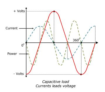
In a capacitor, the current flowing in it depends on the voltage difference across it. An alternating supply allows it to charge when the voltage is increasing above zero, and discharge when the voltage reducing towards zero. **Because** capacitor has almost no internal resistance, and most loads that it is connected to have only very small resistances in series with the capacitor, the charging and discharging currents largely depend on the rate at which the voltage is changing.
