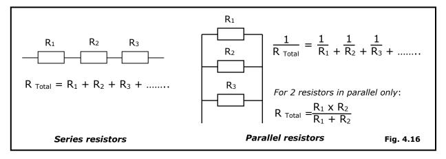
It is not practical to manufacture resistors to every possible value hence "preferred values" are used. These values are such that, when the spread of tolerance limits is considered, the entire range of resistance can be achieved by combinations of series and parallel connections.
