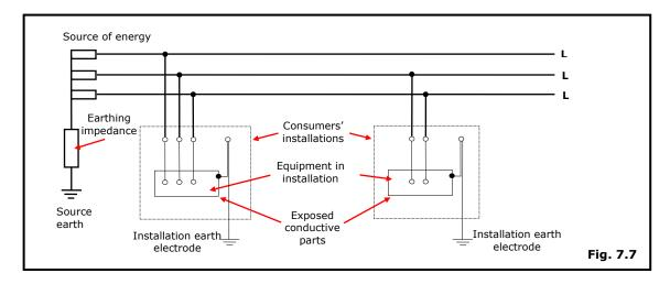
It should be noted that Chapter 54 of the I.E.E. Regulations (17<sup>th</sup> Edition) give complete details of earthing and protective conductor arrangements.
