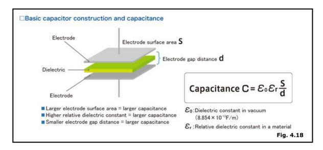
In Fig. 4.19 (below) two plates with area (A) are separated by distance (d) with a dielectric material. When a charge of  $\pm Q$  is applied across the plates an electric field (E) is generated in the region between them. The dielectric material becomes polarised and the resulting field opposes the field of charge on the plates, reducing the total internal field, and increasing the capacitance.
