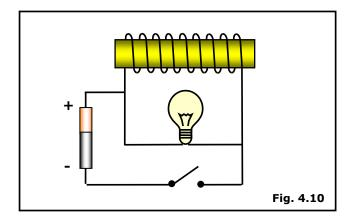
The coil resistance is less than that of the lamp hence, when S is closed, the expectation would be for most of the current to flow through the coil, leaving the lamp to glow very dimly. In reality, when S is closed, the lamp glows brightly and then gets dimmer. When the switch is opened, the lamp glows brightly and then quickly extinguishes.
