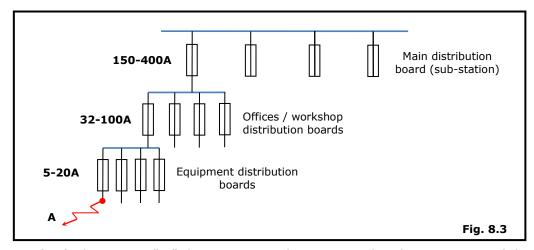
In the event of a fault at point "A" the protection device immediately up-stream of the fault should operate and isolate the faulty circuit. It is desirable that only the upstream device should operate if it is able to clear the fault by itself, hence leaving the healthy circuits unaffected. This is known as **discrimination**.
