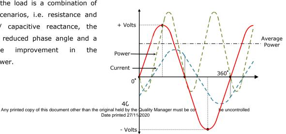
It is accepted that the voltage is the reference quantity hence the following mnemonic may be used to indicate the phase relationship between the current and voltage
