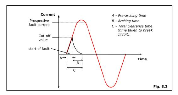
The energy that is allowed through the circuit before the fuse disconnects can be calculated by the formulae  $(I^2.t)$ .
