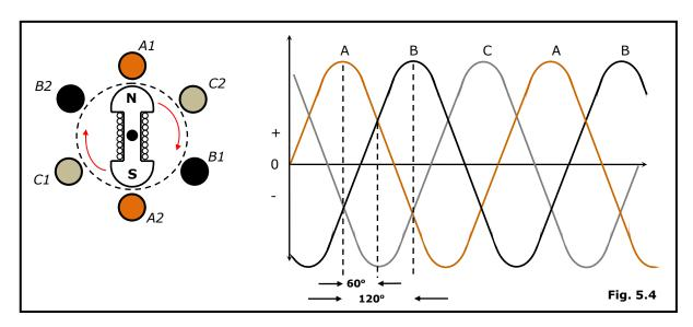
In the generator shown in Fig. 5.4, two more coils, B1-B2 and C1-C2, are added and spaced 120° apart from coil A1-A2, (the colours represent the Regulatory phase identification colours for the UK and Europe). As the magnet rotates voltage is generated in each coil the peaks of which are at 120° intervals as shown in the diagram.
