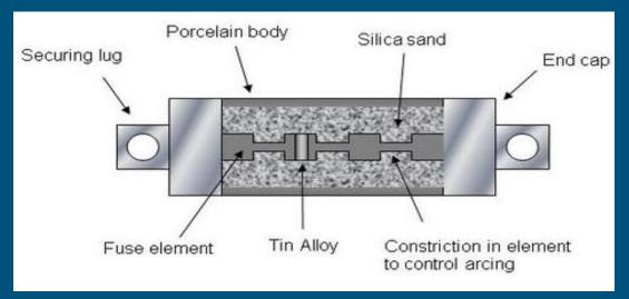
**Fusing element** – Specially shaped elements are used. The shaping of the elements allows for controlled operation of the element during melting by one or more of the constricted (narrow) sections melting and fusing with powder to form globules of high-resistance in the path of the arc, resulting in it being extinguished and insulating the end caps.
