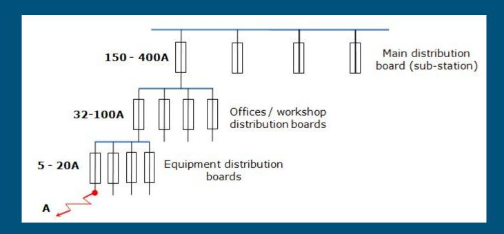
In the event of a fault at point "A" the protection device immediately up-stream of the fault should operate only and isolate the faulty circuit, hence leaving the healthy circuits unaffected. This is known as discrimination.
