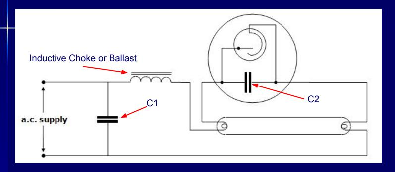
By adding a capacitor (C1) in parallel with the supply we can bring the current and voltage nearer to unity power factor. The capacitor (C2) across the starter is used for RFI suppression.
