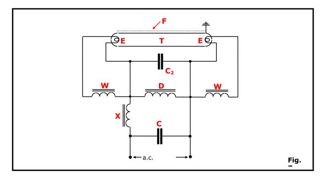
The electrode pre-heating is provided by a small auto-transformer, the primary winding **D** being connected across the lamp electrodes **EE**. A thin metallic strip **F** is attached to the outer surface of the tube and is connected to earth via the lamp caps.
