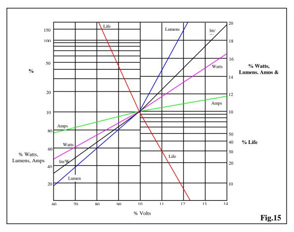
The diagram above, (Fig. 15), shows how the lamp efficacy, life, light output and electrical energy consumed vary with changes in the supply voltage.
