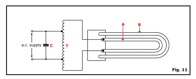
The oxide-coated tungsten electrodes are connected to a step-up auto-transformer, **T**, designed to have a relatively large leakage reactance. When this transformer is on open-circuit, its output voltage is approximately 500V., and this is sufficient to initiate a discharge through the gas. This discharge has a reddish colour however, as the gas discharge increases the temperature, the sodium is vaporised and the discharge changes to monochromatic light.
