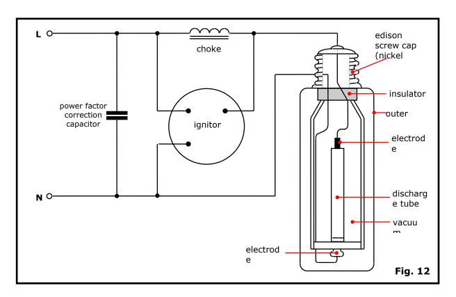
Hot sodium-vapour is highly reactive and would attack conventional arc-tube materials eventually discolouring or destroying them. Also, in order to achieve the high vapour pressure, the coolest section of the arc-tube must be at 750°C therefore the arc-tube is made of sintered aluminium-oxide which is the only material known that is capable of withstanding a sodium-vapour attack. Most high-pressure sodium
