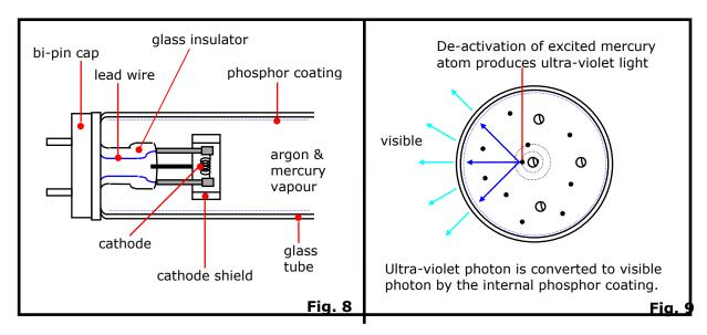
Fluorescent lamps are constructed with a coiled filament at each end of the glass tube (see Fig. 8). A cathode shield, in the form of a metal strip bent into an oval shape, surrounds the cathode and has a number of purposes :-
