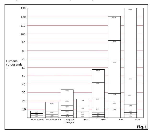
The quantity of light emitted, often the initial lumens, divided by the power input in watts, is known as efficacy and is measured in <u>lumens per watt</u> (<u>lm/W</u>). This is instead of the term efficiency which can only truly be applied when two quantities of the same units are compared.
