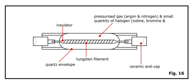
By introducing a small quantity of a halogen into the gas filling, a process called the tungsten halogen cycle occurs. Halogen elements used in this type of lamp include iodine, bromine and chlorine, and under the right conditions their atoms can combine with atoms of other elements without altering their characteristic.
