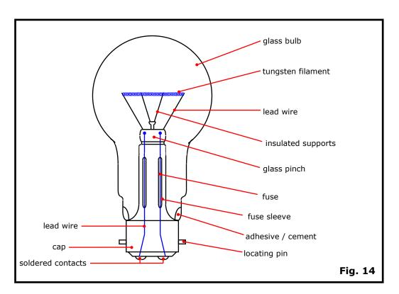
Filament lamps are made in a bewildering variety of sizes, colours and shapes. References should always be made to a manufacturers catalogue if specific details are required. Lamps are frequently used in fittings called luminaries which are designed to provide the required light control. If the luminaire is enclosed, it will be marked to
