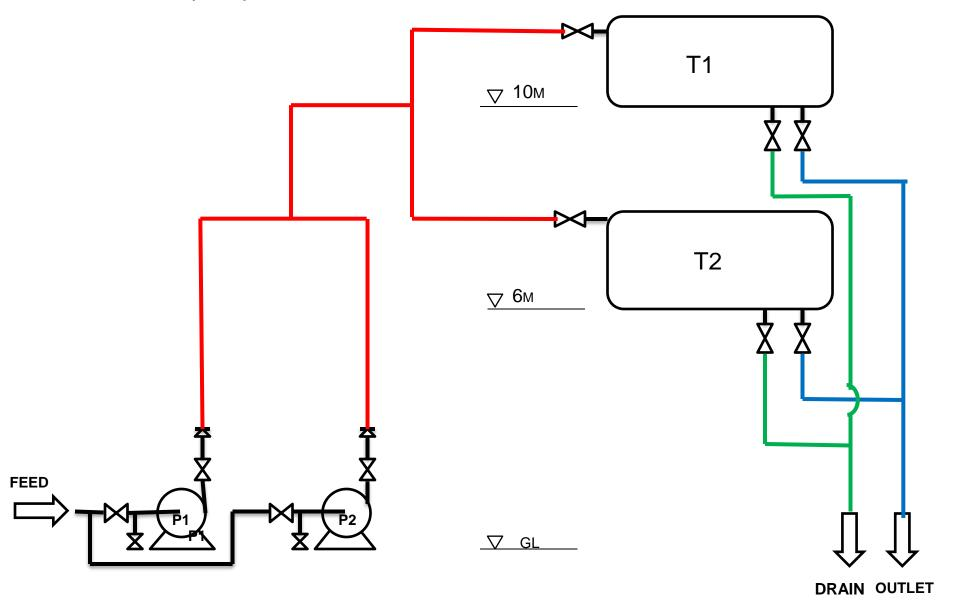
Design a simple piping system to connect pumps to tanks, a common drain and common outlet Line diagram of 2 pump, 2 tank system
