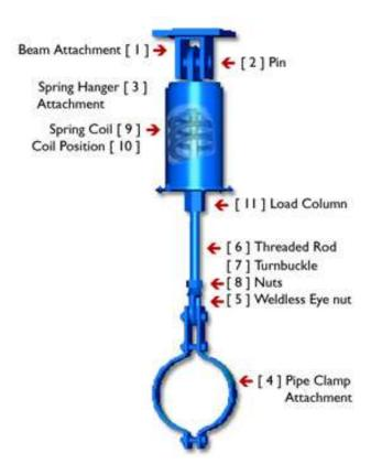
DROP ROD & CLIP ASSEMBLY WITH VARIABLE SPRING UNIT (SUSPENDED TYPE)
