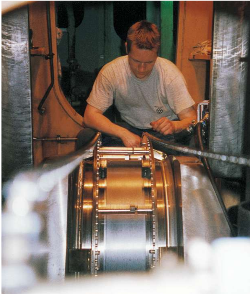
Turning a crankpin journal of a main diesel engine.
