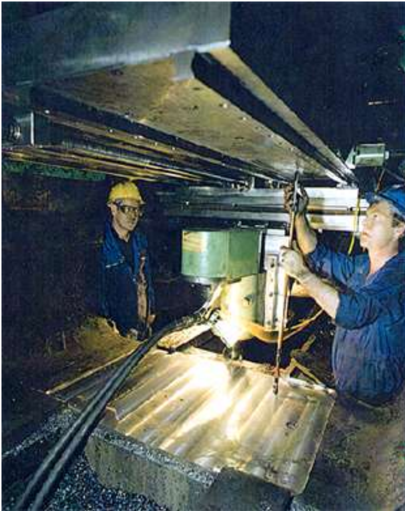
Specifically designed Mill Stand Base Milling Machine. Operator & drive side bases are machined simultaneously
