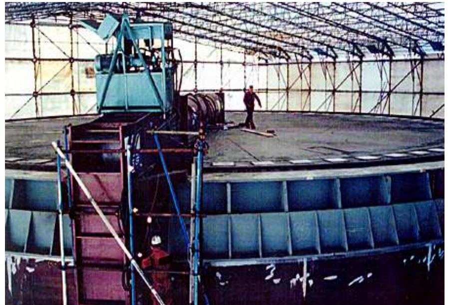
Machining of a Ø26000mm Crane Slew ring surface. 6000kg of material removed during this contract
