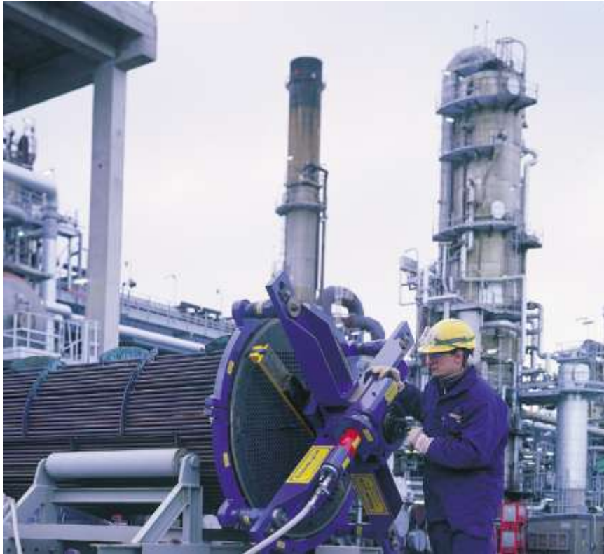
On-site machining of the flange on a heat exchanger.
