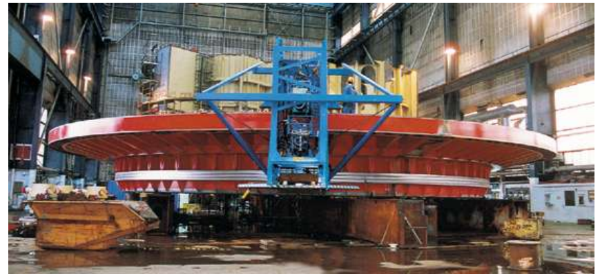
22 m diameter FPSO turret machining in progress. Developed in our R&D Centre.
