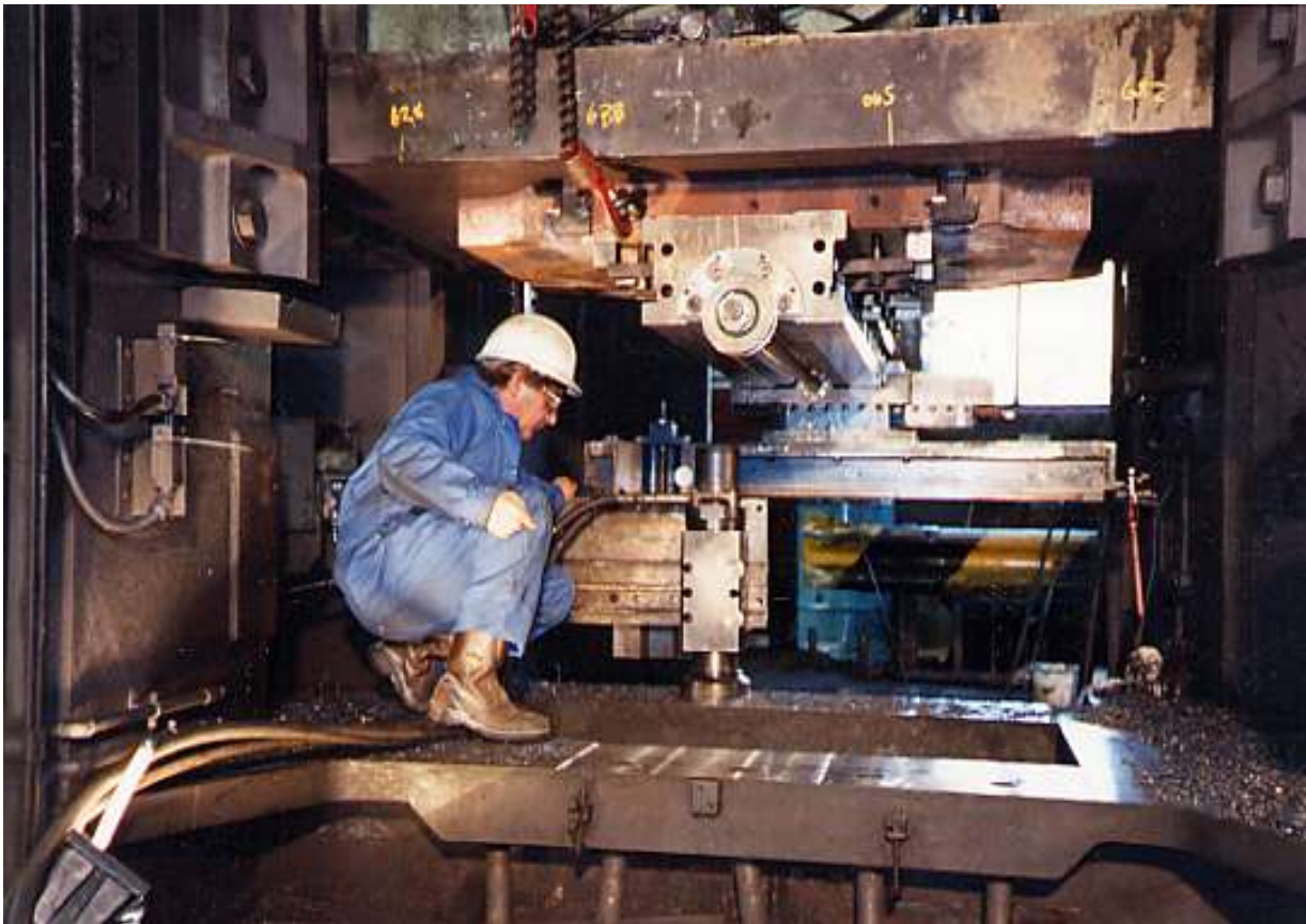
Machining of base plates of automotive press tool
