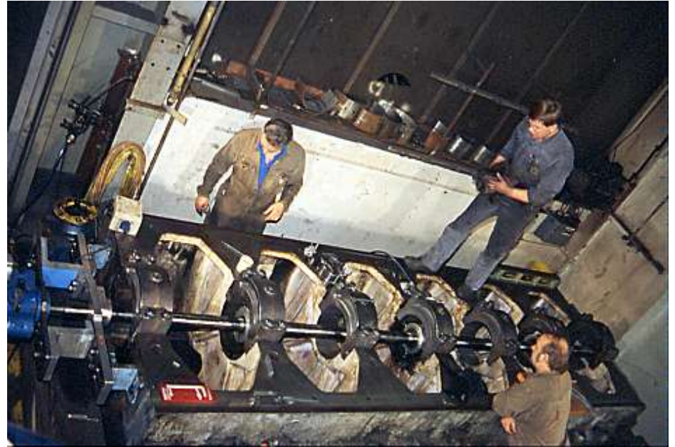
Line boring engine bearing pockets
