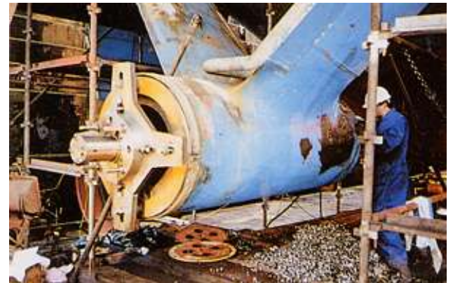
In-Situ boring of an 'A' bracket of a large cable laying vessel
