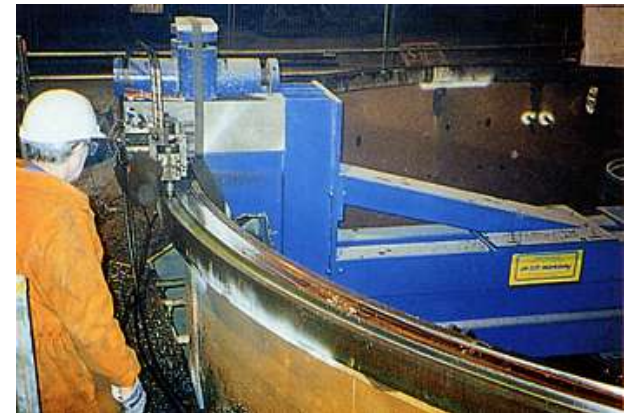
8000mm dia. Flange and seal groove machine of a BOS vessel horizontal joint
