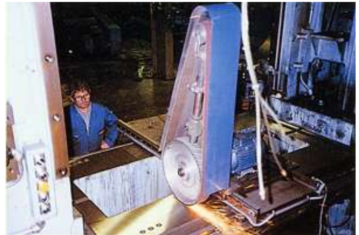
Precision grinding of a 2000mm x 1500mm wide die location bed of a canning press
