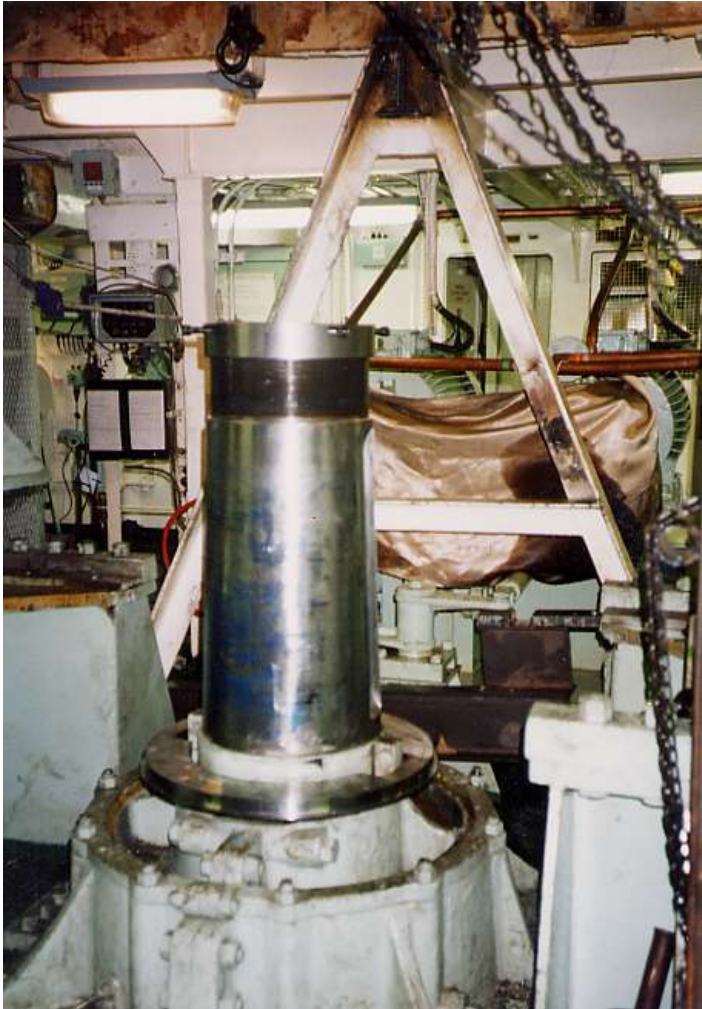
RFA Fort Austin Taper Grinding Rudder Stock
