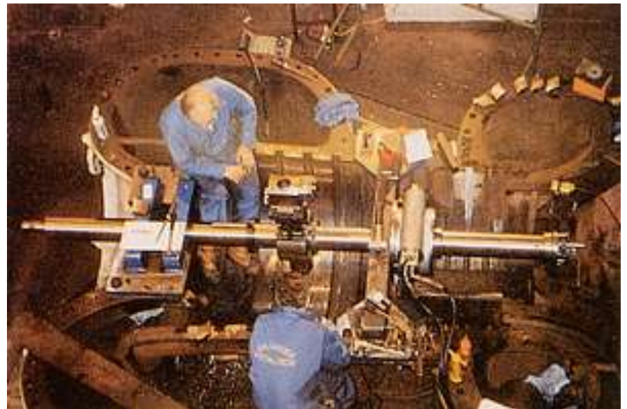
Line boring labyrinth seal groove to a steam turbine casing
