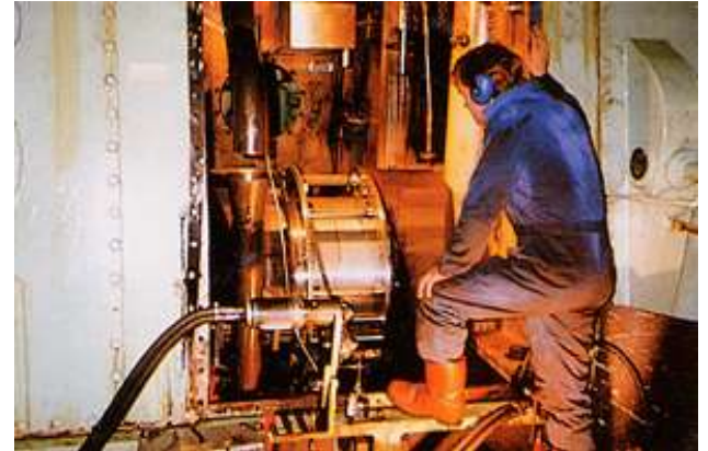
On board machining of a 730mm diameter crankpin journal
