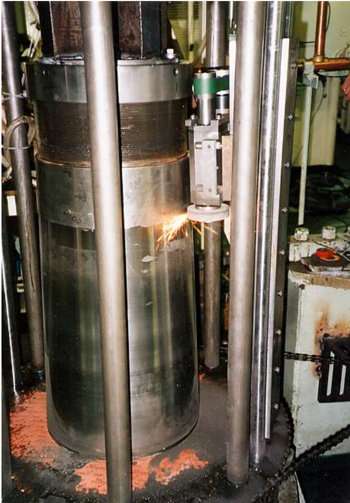
RFA Fort Austin Taper Grinding Rudder Stock
