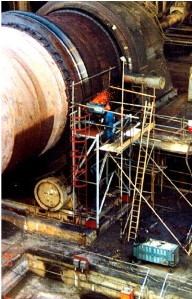
In-situ grinding of a Ø6000 Cement Kiln
