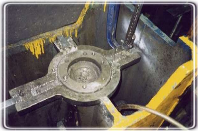
Steel Collar used to assist with the repair
