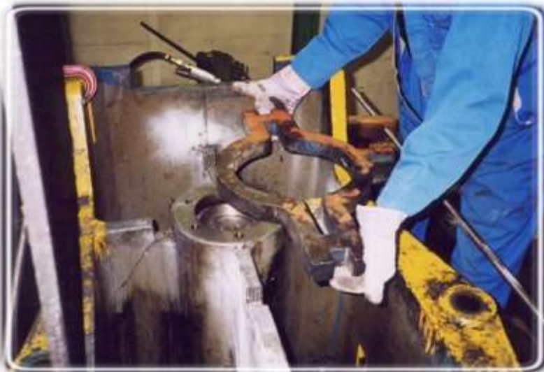
Steel Collar used to assist with the repair
