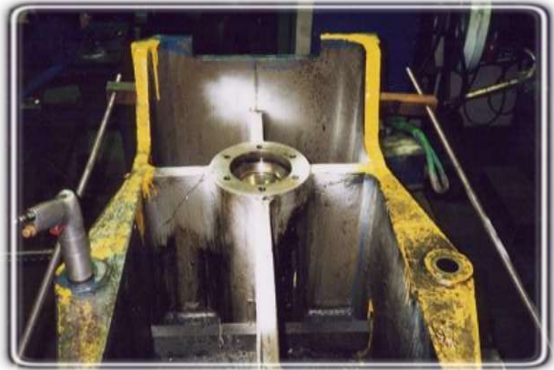
Steel Collar used to assist with the repair
