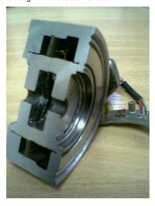
C2 are equal. If an increase of pressure is applied to the H.P side, then the distance D1 will reduce thus changing the capacitance C1, this information is fed to the electronics which will detect the difference in the two capacitance values and convert this into a 4 - 20mA output signal.
