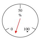
3. If the Indications are the same but either slightly above or below the zero point on the gauge - If the tank was known to be empty this could be due to a zero error on the transmitter. If this was applicable to only one gauge it could be a zero error on that particular gauge.
