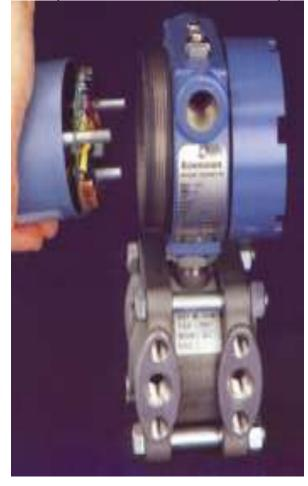
The handset may be connected directly to the transmitter, or it can be connected to part of the wiring loop inside the control panel area. Newer breeds of handsets are capable of storing information on upto 100 individual transmitters. Most standard electronic transmitters can be fitted with replacement smart electronics. The transmitter itself will have push button zero and range adjustment rather than traditional potentiometers.
