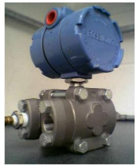
to 4 - 20mA or other suitable output signal. As a standard the supply for electronic transmitters is 24Vdc.
