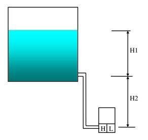
The overall pressure acting on the transmitter is:-H1 + H2. where H2 is static the head pressure, and H1 is the actual level in the tank. This error (effect of H2) may be eliminated suppressing the zero.
