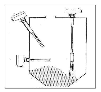
In some systems it is common to see a series of these units mounted up/ into the vessel wall this detects rising and falling product between the sensors, or alternatively the sensor may be suspended into the tank from the top, this is common for high level alarms in large silo's or storage tanks.
