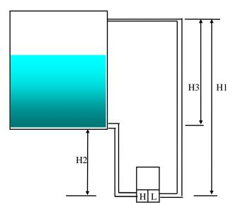
The following diagram shows an example of a suppression/ elevation kit, as fitted to the Foxboro range of pneumatic transmitters:-
