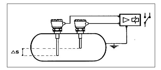
Only about 50mm of conductor at the probe is immersed into the product. The checking of the system merely involves raising the
