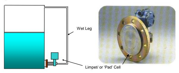
The use of the limpet cell is not restricted to closed vessels only, it may also be used on open tank installations or it may be used to measure density if the level in the tank is kept constant.
