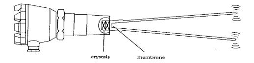
forks the natural vibration is dampened or stopped, this is detected within the electronics and a switched output may be generated to create or initiate an alarm. The diagram below shows typical uses of this system:-
