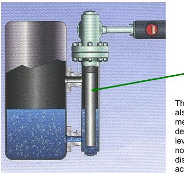
These devices can be used to measure level from approx 10" to about 15 ft, this being determined by the length of the displacer tube.
