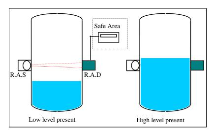
As the diagrams show when the radiation beam is interrupted by the product, no radiation hits the detector, and as a result the output to the electronics would initiate a high level alarm warning. In addition to alarm use, this system may also be used for indicating the actual level as the next diagrams show:-
