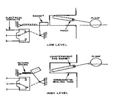
These devices are limited to the point at which the are inserted into the tank and the length of the connecting arm.
