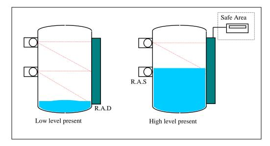
In the diagrams above the first would show a low level near 5%, whereas the second diagram would be indicating a level in the region of 60%, therefore the reduction of radiation intensity creates a higher output level and level reading.
