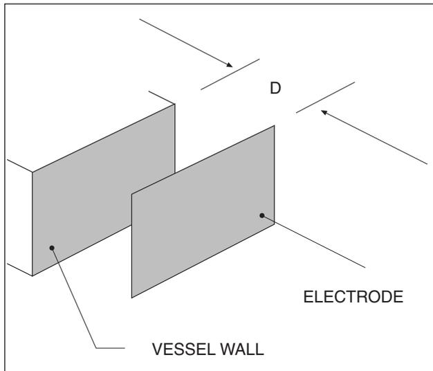
The dielectric constant is a numerical value on a scale of 1 to 100 which relates to the ability of the dielectric (material between the plates) to store an electrostatic charge. The dielectric constant of a material is determined in an actual test cell. Values for many materials are published by the National Institute of Standards and Technology.
