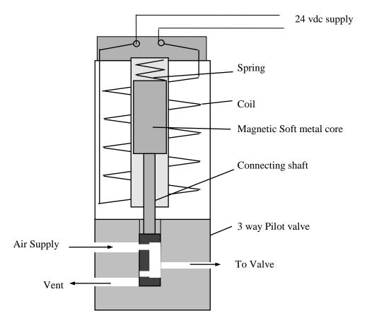
From the above diagram, the basic solenoid consists of a coil, soft metal core connected to a 3 way pilot valve.
