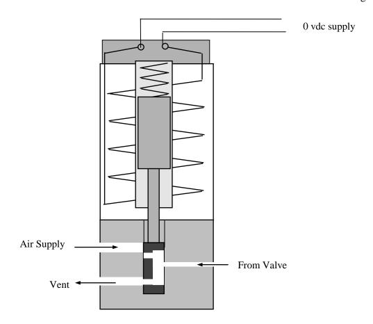
The previous diagram shows the solenoid in its de-energised state. The small spring is used to force the metal core to its original position, with this movement happening in micro-seconds. The supply is now blocked off, whilst the air to the valve is allowed to backtrack through the solenoid and via the vent to atmosphere.
