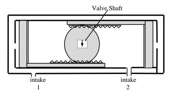
In some cases it may be required that an auto return operation is needed such as for shutdown valves, in this case the supply air will only be fed via intake 2 with intake 1 being used as an exhaust and heavy duty springs would be fitted into chambers 1 and 2, as shown below:-
