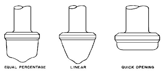
Valve plug shapes to produce the three common flow characteristics.
