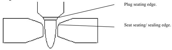
The most common materials used for plug and seats are stainless steel, Stellite, stainless steel with Stellite coating, or Monel. Stellite or Monel material tends to be used on particularly corrosive natured substances, whilst the stainless steel option is probably best suited for general purpose.
