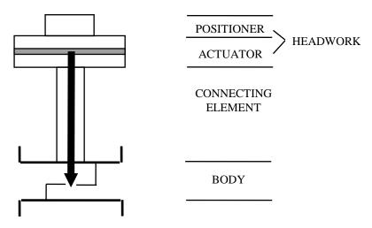
The Positioner- this is an optional unit used to accurately position the correcting element. This usually incorporates a feedback mechanism which senses the input in relation to the actual position of the correcting element.
