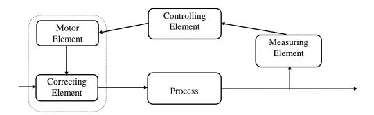
As can be seen in the above diagram the combination of the Motor and correcting elements are normally referred to as the control valve. In terms of parts of the control valve the motor element combines the *positioner* and *actuator*, whilst the correcting element is the device used to manipulate or start/ stop or control the flow.
