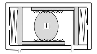
The diagram left shows the springs fully extended with the valve in the closed position.
