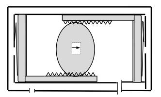
This type of operation is typical of the types of valves manufactured by Norbro and Hytork, their specific applications tend to be shutdown or batch control application. In some instances the top of the valve shaft can be modified to accommodate a proximity position sensor so that a switched signal may be generated that may be used by DCS control systems or panel indications.
