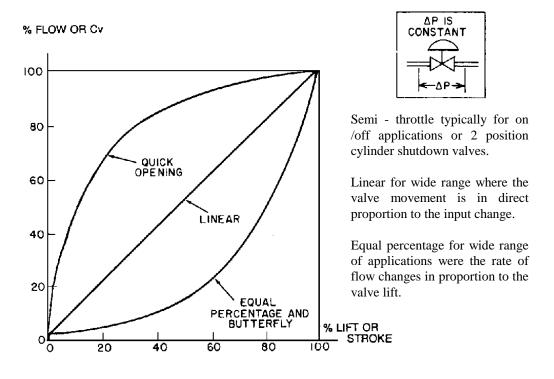
Inherent flow characteristics: quick-opening, linear, and equal percentage.
