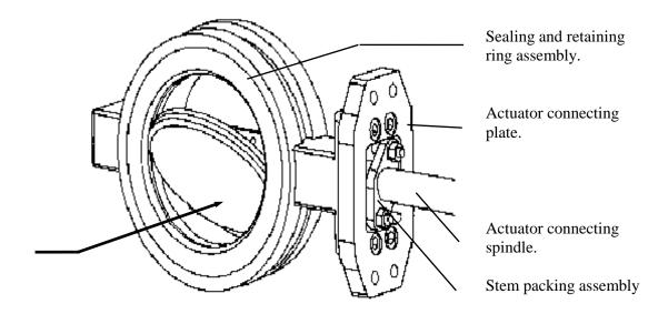
The operation of this valve requires a rotary actuator, as the butterfly is required to be turned through 90 degrees, although a piston actuator and lever mechanism can be used for large applications.
