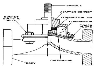
The Saunders valve or diaphragm valve consists of a metal weir body and flexible diaphragm. The next diagram shows the basic parts diagram of this type of valve:-
