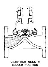
It is opened and closed by moving the diaphragm closer to or away from the weir, this is done via spindle which is connected to the valve actuator and the other end to the diaphragm.
