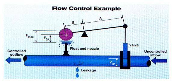
A mechanical flow controller manipulates the valve to maintain the downstream flow rate in spite of the leakage. The size of the valve opening at time t is V(t). The flow rate is measured by the vertical position of the float F(t). The gain of the controller is A/B. This arrangement would be entirely impractical for a modern flow control application.
