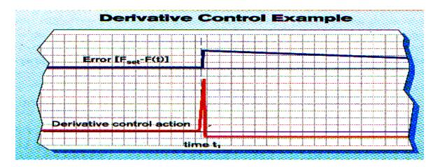
The blue trace on the chart shows the error between the process variable F(t) and its desired value Fset. The derivative control action in red is the time derivative of the difference. Derivative control action is zero when the error is constant and spikes dramatically when the error changes abruptly.
