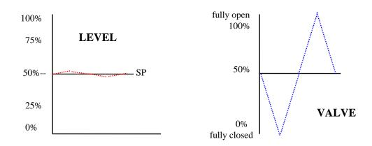
This time it can be seen that the proportional band is only about 4%, so now 1 unit input creates an output of 100%, a gain of 25.
