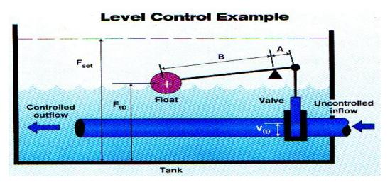
The same mechanical controller now manipulates the valve to shut off the flow once the tank has filled to the desired level Fset. The controller gain of A/B has been set much lower, since the float position now spans a much greater range.
