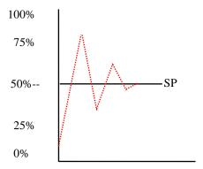
The above diagram shows the combined effect of PID acting together in response to a process change, and represents the ideal response.
