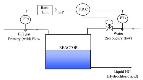
In the above example, as the HCl gas flow changes the water flow is ratio'd to it to maintain a percentage balance in the reactor so that the make-up of the Liquid HCl out remains the same.
