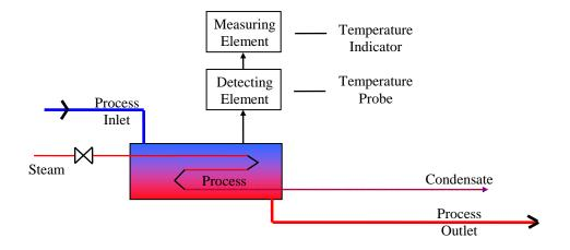
To change the temperature the process operator would have to manually adjust the position of the hand valve until the desired temperature was reached.
