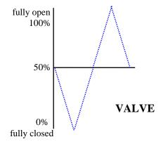
From the diagram above you can see that as the level rises above the setpoint the control valve closes by an equal amount. This system is said to have a *proportional band* of 100%, because the level has to go from empty (0%) to full (100%) to get the valve to move by the same percentage amount. If the supply to the tank was quite fast and therefore the changes were rapid, we would need the system to respond differently, as the next diagram shows:-
