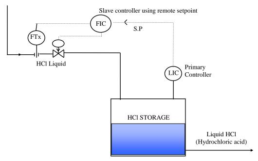
In this system the level in the storage tank needs to be maintained, so the introduction of the cascade system means that the flow into it may be kept at a steady flowrate rather than having the control valve going fully open to fully
