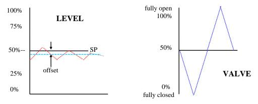
In some systems a small degree of offset may be acceptable. However in others it may not and therefore needs to be reduced or eliminated. This is done by adding a second mode of control to proportional. The mode to be added is *Integral Action*.
