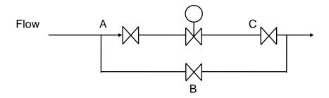
To operate the bypass, valve B should be opened first. Then isolate valves A & C. Any pressure needs to be carefully vented and the control valve can either be removed or stroke checks carried out. Returning the system to normal is the reverse of the isolation procedure. As a guide, remember Bypass first and last.
