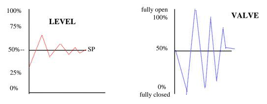
Unfortunately what this system does not do is take into account the rate of process change. For example temperature processes tend to be slow, whereas pressure, level and flow tend to change more rapidly. Because of this it is possible to lose control quite quickly with a fast reacting process. To overcome this problem the final mode of control is added, this is called Derivative action.
