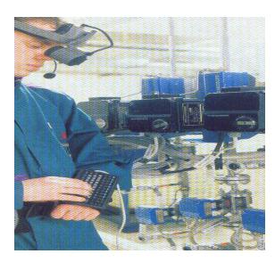
In the following example, the operator can view and operate the plant from a head mounted LCD display unit and arm mounted control pad. With this technology the operator can operate the plant from anywhere with communication range
