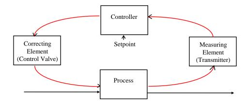
The next point to consider is what would happen if the measuring element developed a fault. Quite simply the controller would respond to the error as if it where the actual condition and this is impractical as will be explained in later sections.
