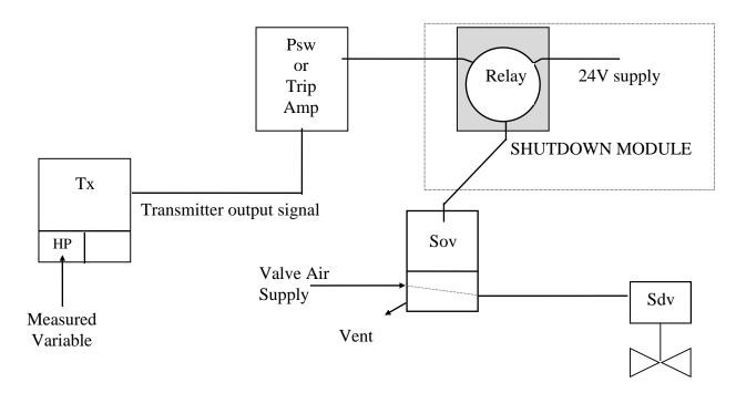
The above diagram represents a simple shutdown system using a relay to provide the logic function as to whether or not an output is required dependant upon the input state. The above system consists of a single input, and gives a single output. The diagram below displays this information as a simple ladder diagram. The pressure switch acts as input 1.
