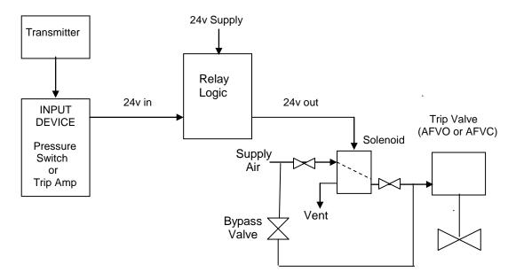
The solenoid is by-passed by opening the by-pass valve before closing valves A and B. This ensures that even when the solenoid de-energises, supply air to the trip valve is maintained via the by-pass facility.
