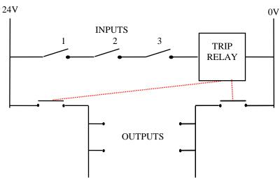
In reality 'it is the relay contacts that are wired in series not the actual inputs'. Each input is assigned its own relay, which contain 2 sets of normally open contacts. One set is used to operate / form the input switch for an alarm circuit, while the second set form the series chain to the final trip relay. As shown in the next diagram:-
