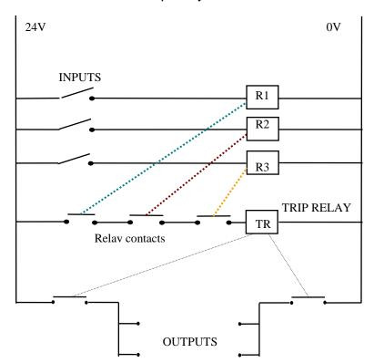
From the diagram previous, the relays used for R1, 2, 3 would be 8 pin, whilst the trip relay would be an 11 pin relay. A variation to the above could be the 2 out of 3 input shutdown module, this would be configured as shown in the next diagram:-
