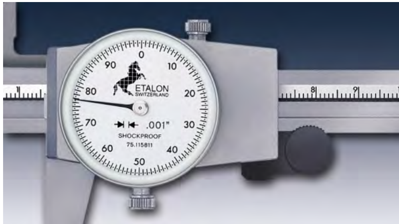
Figure 8 Close up of the dial. Note that there are 100 divisions in one revolution. The resolution is 0.001 inch (courtesy Tesa group).
