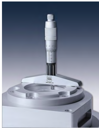
Figure 71 Using a depth micrometer (courtesy Tesa Group)
