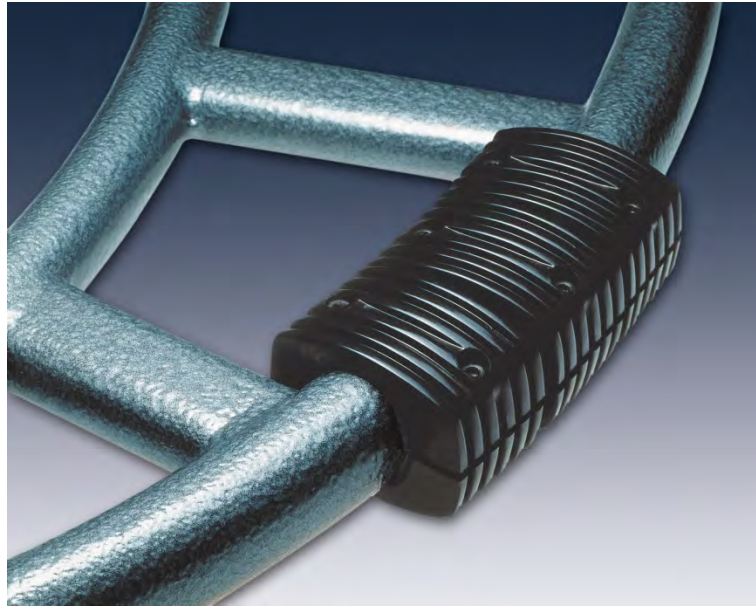
Figure 57 Some micrometers are fitted with thermal insulation to prevent the operators hands heating the micrometer frame (courtesy Tesa Group)
