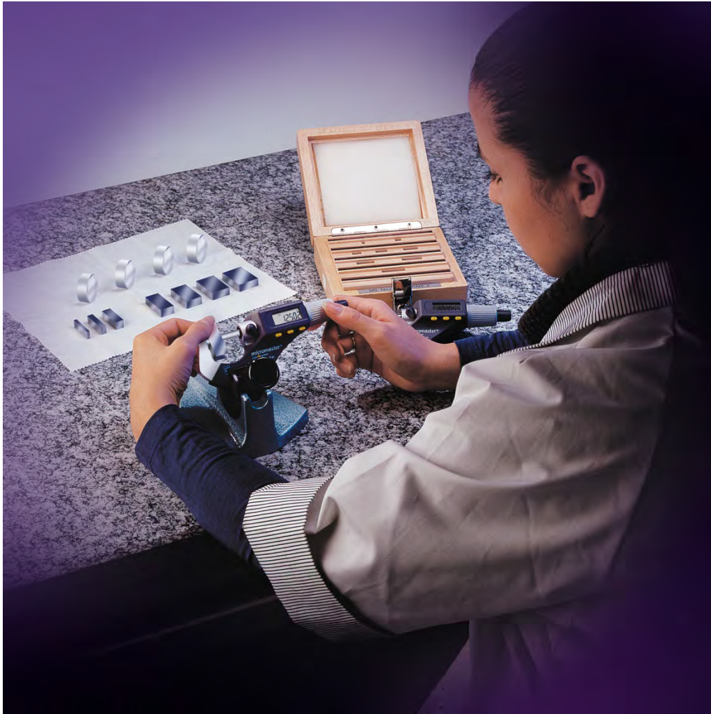
Figure 63 Calibrating a micrometer (courtesy Tesa Group)
