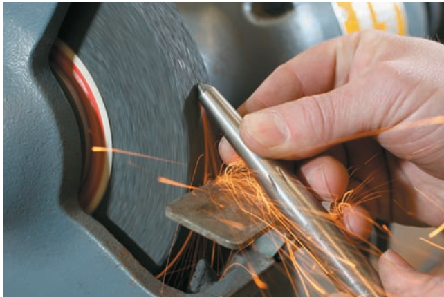
Figure B-165 This punch is being correctly sharpened to produce a 90-degree angle for use as a center punch. It must be rotated while being ground. A sharper angle of 60 degrees may be ground to produce a prick punch.
