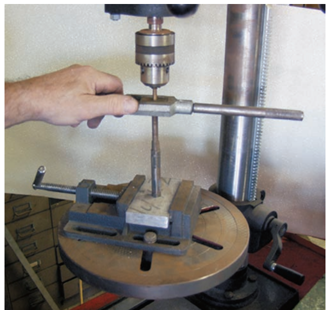
Figure B-112 Using the drill press as a reaming fixture.
