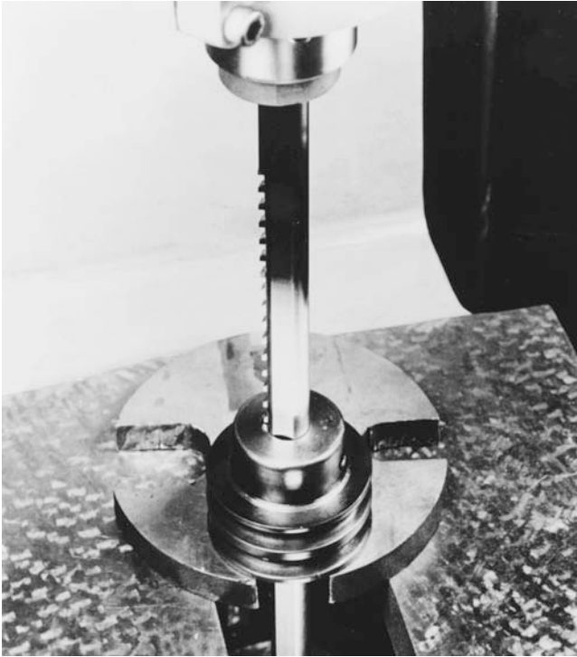
Figure B-17 Production push broaching without bushing or shims ( The duMont Company, LLC ).
