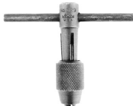
Figure B-135 T-handle tap wrench.
