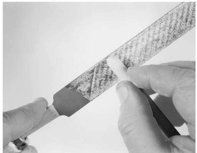
Figure B-95 Using chalk on the file to help reduce pinning.
