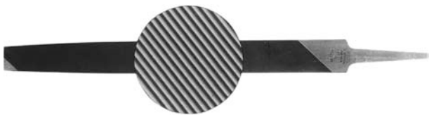
Figure B-79 The lathe file has a longer angle on the teeth to clear the chips when filing on the lathe.
