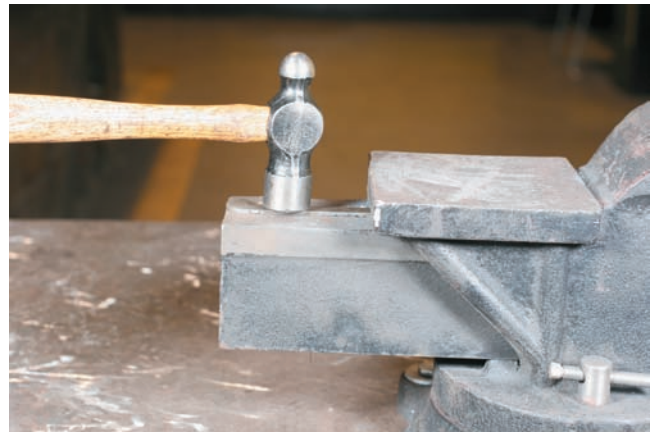
Figure B-24 Never hammer on the slide bar of a vise. This may crack or distort it.
