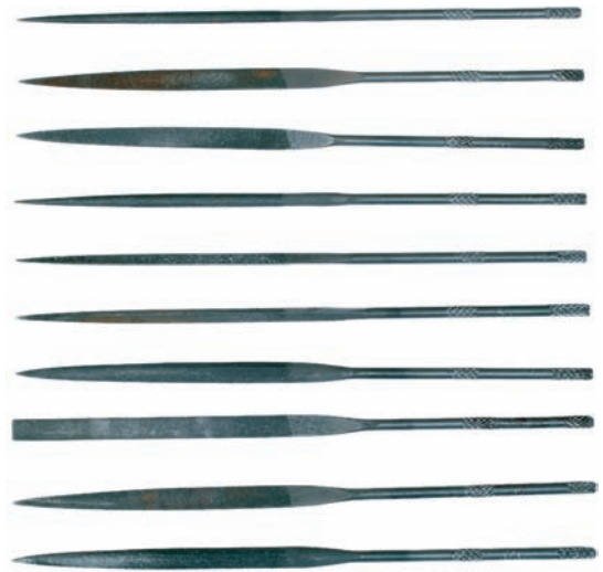
Figure B-88 Set of Swiss pattern files. Since these small files are very delicate and can be broken quite easily, great care must be exercised in their use.
