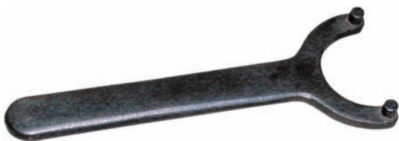
Figure B-51 Fixed face spanner.
