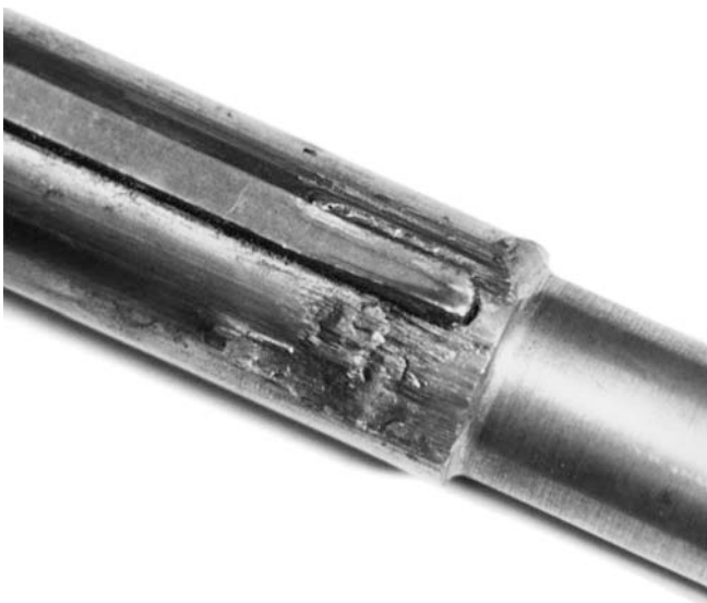
Figure B-10 This shaft had just been made by a machinist and was forced into an interference-fit bore for a press fit. No lubrication was used, and it immediately seized and welded to the bore, which was also ruined.
