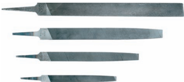
Figure B-74 Files are made in several different lengths.
