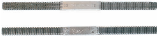
Figure B-92 Thread files.
