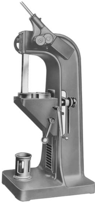
Figure B-2 Simple ratchet floor-type arbor press ( Dake Corporation ).
