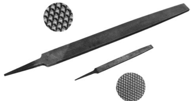
Figure B-76 These two files are both bastard cut, but since they are of different lengths, they have different coarsenesses.
