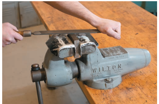
Figure B-98 Proper filing position.
