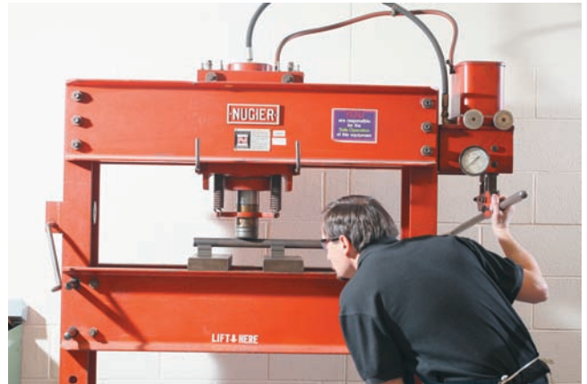
Figure B-19 Pressure being applied to straighten shaft.
