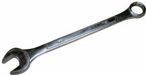
Figure B-47 Combination wrench.
