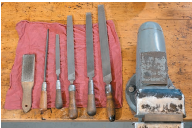
Figure B-93 Files should be kept neatly arranged so that they will not strike one another and damage the cutting edges.
