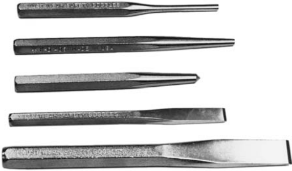
Figure B-64 Common chisels and punches used by machinists. Top to bottom: pin punch, drift punch, center punch, small flat chisel, and large flat chisel.
