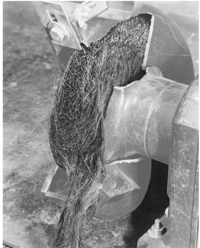
Figure B-167 The force and speed of this action was such that the operator's head was jerked suddenly into the guard. Note that the cast aluminum guard was shattered as a result of the impact.
