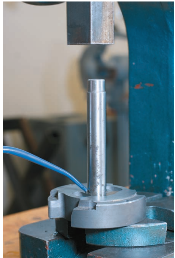
Figure B-11 Mandrel being lubricated and pressed into part for further machining.
