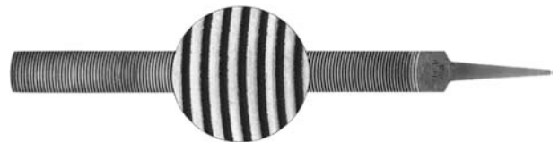
Figure B-90 Curved tooth files are used on soft metals.
