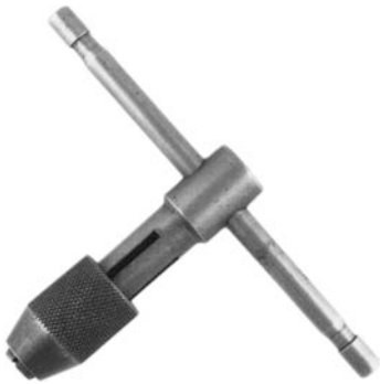
Figure B-58 T-handle tap wrench.
