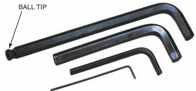
Figure B-55 Socket head wrench.
