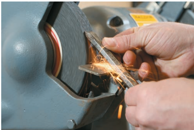
Figure B-166 Flat chisel being ground to produce a 60-degree angle.
