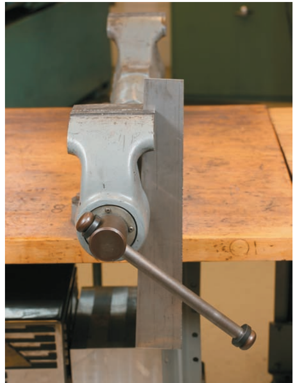
Figure B-20 When long work is clamped in the vise vertically, it should clear the workbench.
