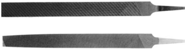
Figure B-77 Blunt and tapered file shapes.
