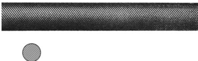
Figure B-87 Round files are used to file a small radius or to enlarge a hole.
