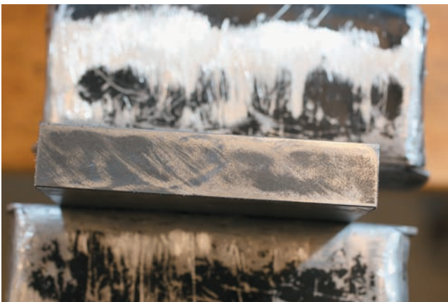
Figure B-97 The crosshatch pattern shows that this piece has been filed from two directions, resulting in a flatter surface.
