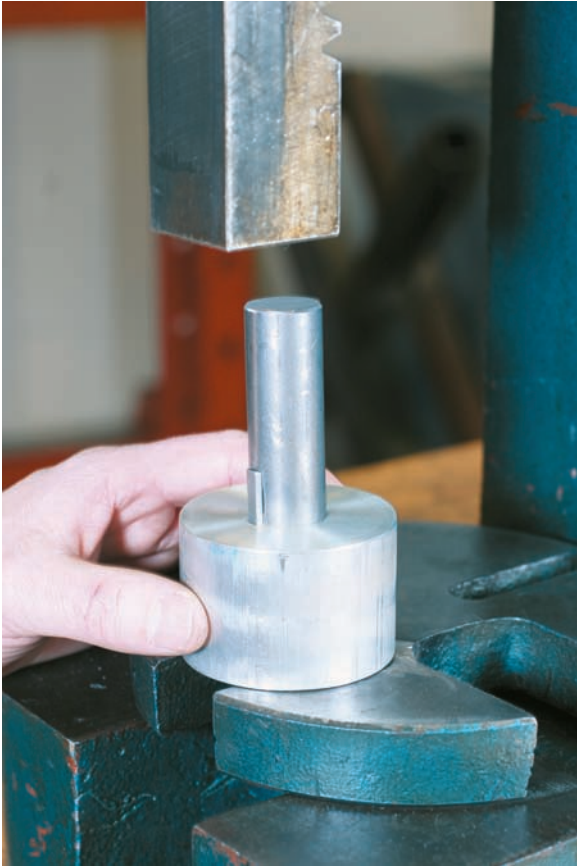
Figure B-9 Chamfer on key helps in alignment of parts being pressed together.
