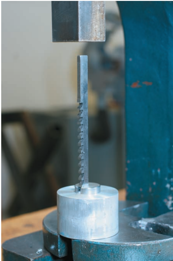
Figure B-15 Broach with guide bushing placed in arbor press that is ready to be lubricated and have the first pass performed.
