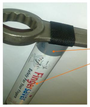
Inspect entire shell for cracks, excessive wear and damage caused by possible hammer strikes
