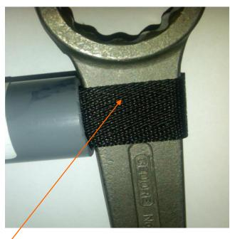
Attach the flogging (slogging) spanner to the Fingersaver using the holding strap.
