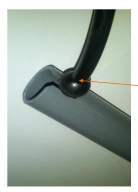
Inspect tensioner for cracks, excessive wear and possible damage caused due to exposure to aggressive liquids
