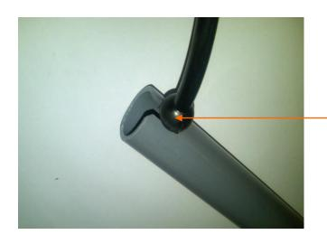
Pulling the tensioner at the back end of the Fingersaver results in the secure attachment of the spanner to the Fingersaver.
