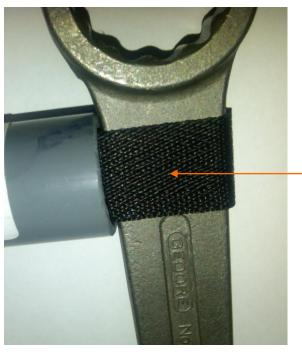
Inspect holding strap for excessive wear, damage caused by possible hammer strikes and tears. Slight fraying is acceptable.
