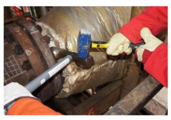
Available in two lengths 350mm and 900mm which allows safe usage for one to two persons.
