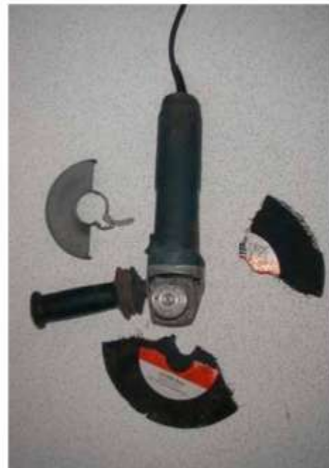
Angle grinder and disintegrated disk
