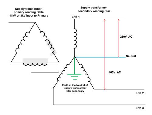
Example of THREE-PHASE TRANSFORMER using Delta/ Star, primary to secondary CONNECTION used for supply transformer.
