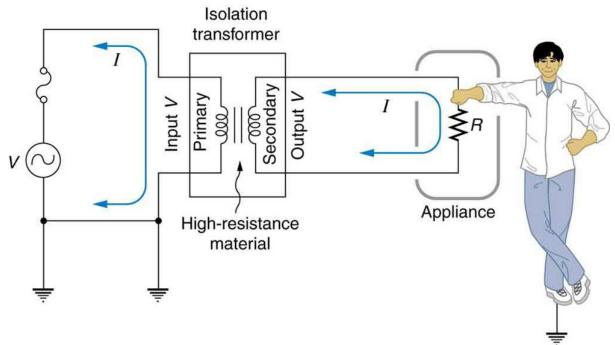
Operator touches Live but current will not flow through his / her body (no electric shock) as there is no return path to the source of the supply on the secondary.
