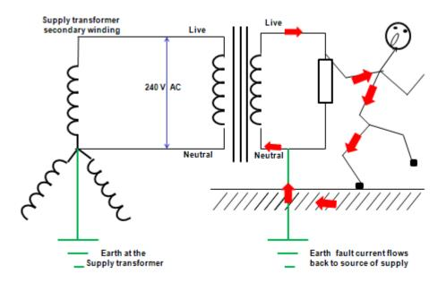
Operator touches Live and current flows through the operator, through the earth (in this case via his or her feet) and returns to the transformer secondary winding via the earth on the transformer neutral.
