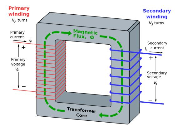
The voltage from the secondary winding is dependent on the ratio of the number of turns on the primary winding compared to the number of turns on the secondary winding.
