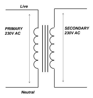
On the Primary winding the Neutral is held a zero volts due to the Neutral being connected to Earth at the Star Point of the secondary in the supply transformer.
