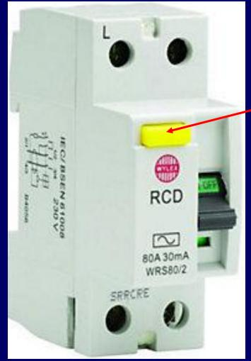
Where an RCD has an integral test device (test button), it should be tested at six-monthly intervals.
