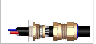
2. Locate the detachable armour cone (C) into the recess of the entry component. Pass cable through entry component evenly spacing the armour around the cone
