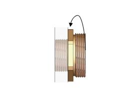
**3.** Locate the detachable armour cone (C) into the recess of the entry component. Pass cable through entry component evenly spacing the armour around the cone.
