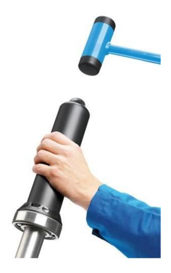
Bearings less than 50 millimetres (mm) in diameter may be mounted by using a bearing driver if the races are installed with a light interference fit. Driving tools consist of a metallic tube, polymer impact rings and a dead blow hammer. This type of tube driver can be used with bushings and oil/grease seals. It is important to use the proper sleeve and impact ring size and ensure the bearing does not become misaligned while being seated.
