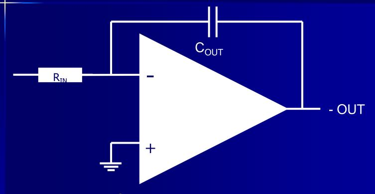
The integrator Op-amp produces an output voltage that is both proportional to the amplitude and duration of the input signal
