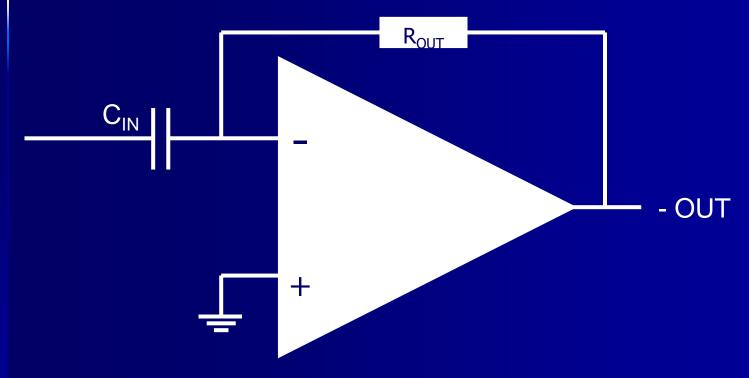
By reconfiguring the feedback loop again this time putting a capacitor on the input, the amplifier will perform the mathematical function of Differentiation.
