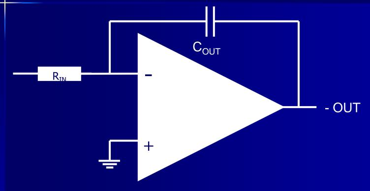
By reconfiguring the feedback loop to incorporate a capacitor from the output, the amplifier will perform the mathematical function of integration.
