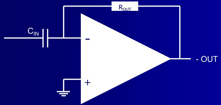
The Derivative amp produces an output which is directly proportional to the input's rate-of-change with respect to time. The faster the change to the input, the faster the output change in response.
