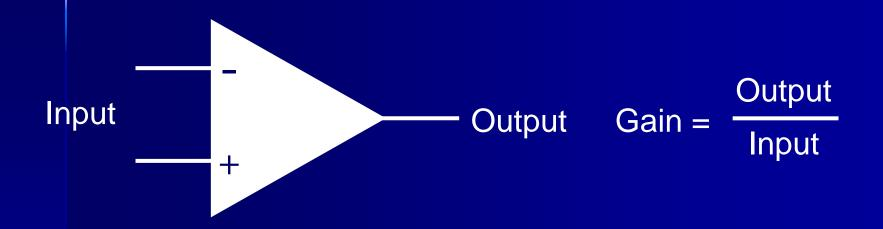
In open-loop gain "no feedback" (i.e. no connection between the output of the op-amp and any of its inputs), the op-amps data sheet specifies that the gain of the op-amp when used in 'open-loop' mode would have an infinite gain.
