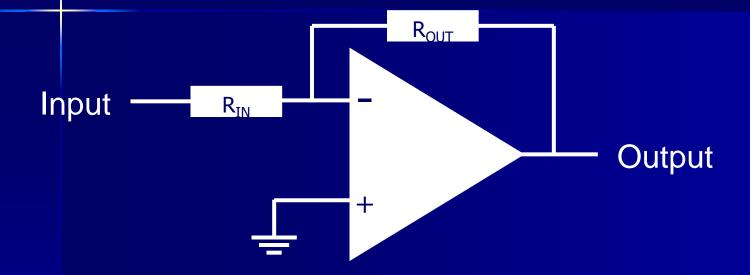
By utilising the Inverting input of the amplifier any sample fed back will be in anti-phase to the original signal and the gain will be proportional to the output / input resistor ratio.
