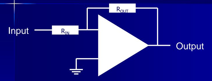
Connecting the output to the input via resistors we can feed a portion of the output back to the input, this will reduce the gain of the amplifier but will give us more control of the output. The ratio  $R_{OUT} / R_{IN}$  of the resistor values will now dictate the gain of the amplifier.
