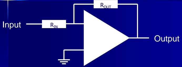
Feedback' means adding a fraction of the output signal to the input signal. When this fraction is returned in phase (in step) with the input signal, it is called 'positive feedback'. When it is out of phase with the input signal, it is called negative feedback.
