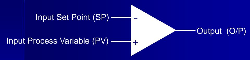
Compares two inputs and gives the output proportional to the difference between the two signals (error).
