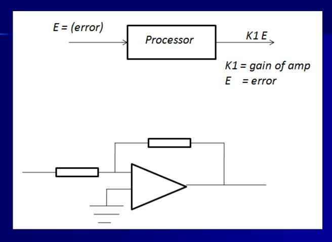
The Proportional Op-amp produces an output voltage that is proportional to the amplitude of the input signal
