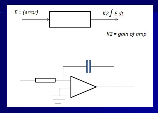
The Integrator Op-amp produces an output voltage that is both proportional to the amplitude and duration of the input signal
