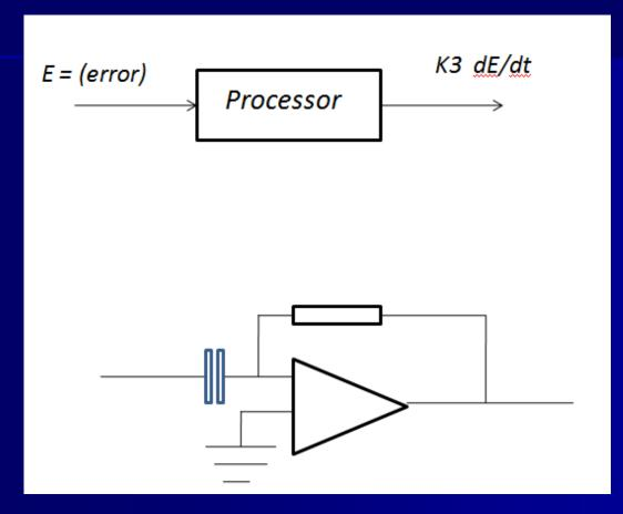
The Derivative Op-amp produces an output voltage that is proportional to the rate of change of the input signal over time
