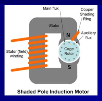
The **shaded-pole motor** is the original type of AC single-phase induction **motor**, dating back to at least as early as 1890. A **shaded-pole motor** is a small squirrel-cage **motor** in which the auxiliary winding is composed of a copper ring or bar surrounding a portion of each **pole**.
