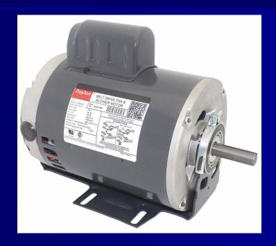
A **Capacitor Start Motor** is a single phase Induction Motor that employs a capacitor in the auxiliary winding circuit to produce a greater phase difference between the current in the main and the auxiliary windings.
