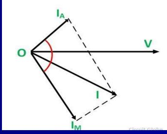
The motor has a cage rotor and two windings on the stator. They are known as the main winding and the auxiliary or the starting winding. The two windings are displaced on the stator by 90 degrees. The capacitor  $(C_S)$  is connected in series with the starting winding by a centrifugal switch  $(S_C)$  which will disconnect the capacitor when the motor reaches full speed.
