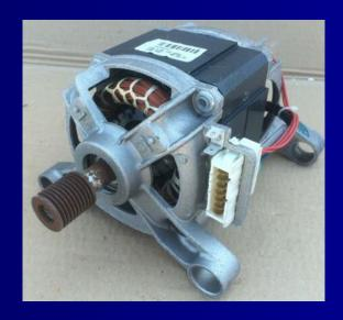
This motor is essentially a DC series motor that due to its design of utilising a commutator to supply current to the armature or rotor, the AC supply will have the same effect on direction of rotation. When the AC stator field windings are alternating so is the rotor field hence Flemings left hand rule will apply.
