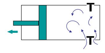
All work on a linear or alternating movement simple & sturdy can pump high viscosity liquids at high pressures
