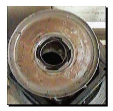
Vertical multistage pumps with pressed impellers do not exhibit the same failure mode as cast components.
