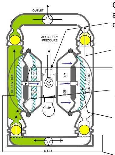
One-moving-part air valve directs air supply to back side of diaphragm
