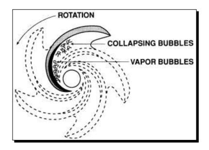
Can be caused by gas or air entrained in the pumped liquid or by a phase change due to pressure fluctuations as the liquid passes through the impeller
