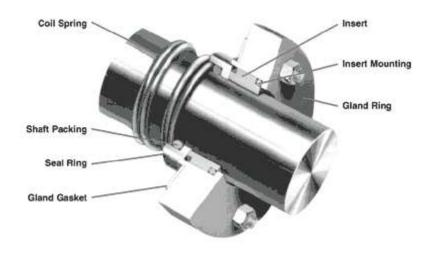
Fig. 9 A Simple Mechcanical Seal
