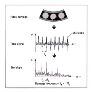
Impacts are created as a rolling element collides with a damaged area.
