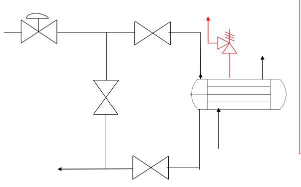
The extra "hand" valves enable us to isolate and remove the heat exchanger without stopping the process.
