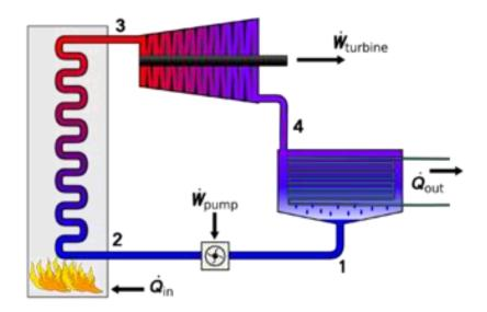
Flow diagram of the four main devices used in the Rankine cycle:
