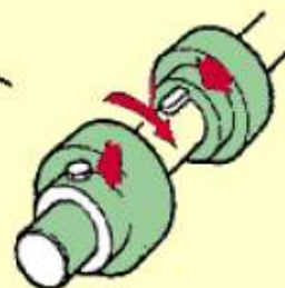
Key and Grub Screw (projection hazard)
