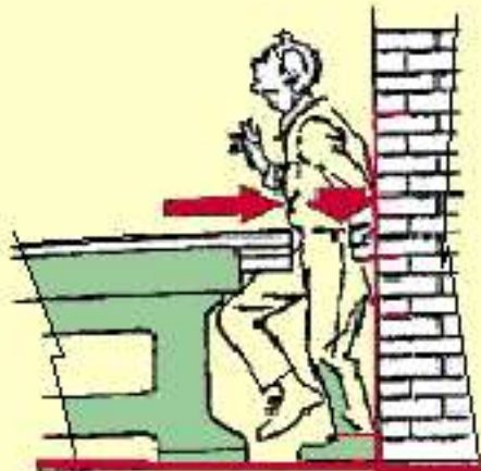
Between moving part of machine and fixed structure (wall)
