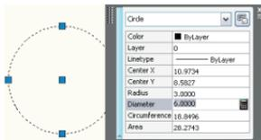
The new Quick Properties tab in the Drafting Settings dialog box provides additional control.
