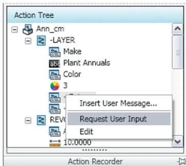
**TIP** Macros don't understand dialog boxes except for the Layer Manager and Properties dialog boxes. All other commands with dialog boxes need to be run at the command line, with a dash [-] in front of the command. For example: -HATCH. The macro can get you into a dialog box, but you will need to enter any information and exit manually.
