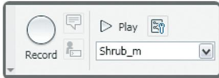
The Action Recorder records actions from the command line, toolbars, ribbon panels, pull-down menus, the Properties window, the Layer Properties Manager, and the Tool palette.
