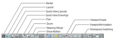
**TIP** Check out the new Hide XREF Scales option added to the VP Scale list.
