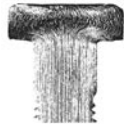
Metal flow lines of a cold-headed product.
