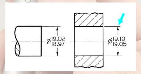
In single-line note form, the low limit precedes the high limit separated by a dash
