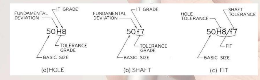
They are a set of tolerances that varies according to the basic size and provides a uniform level of accuracy within the grade.
