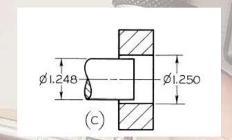
Minimum air space is 0.002". This is the allowance and is always positive in a clearance fit
