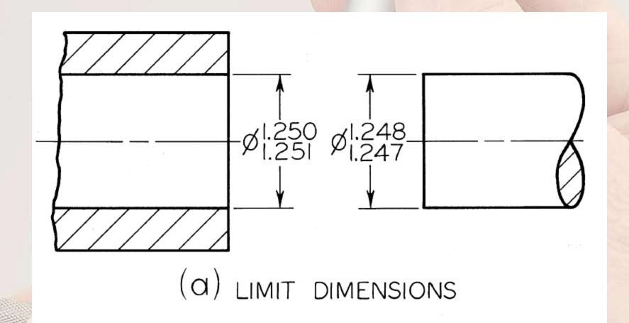
The Tolerance is 0.001" for the Hole as well as for the Shaft
