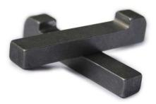
Gib Head Keys are available in metric and inch sizes. Metric sizes are made to DIN 6887 / ISO 2492 and Inch sizes are made to BS 46 Part 1. They are made in key steel with a minimum tensile strength of 55KG/mm or stainless (to order).
