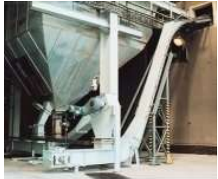
En-masse elevator handling fly ash
