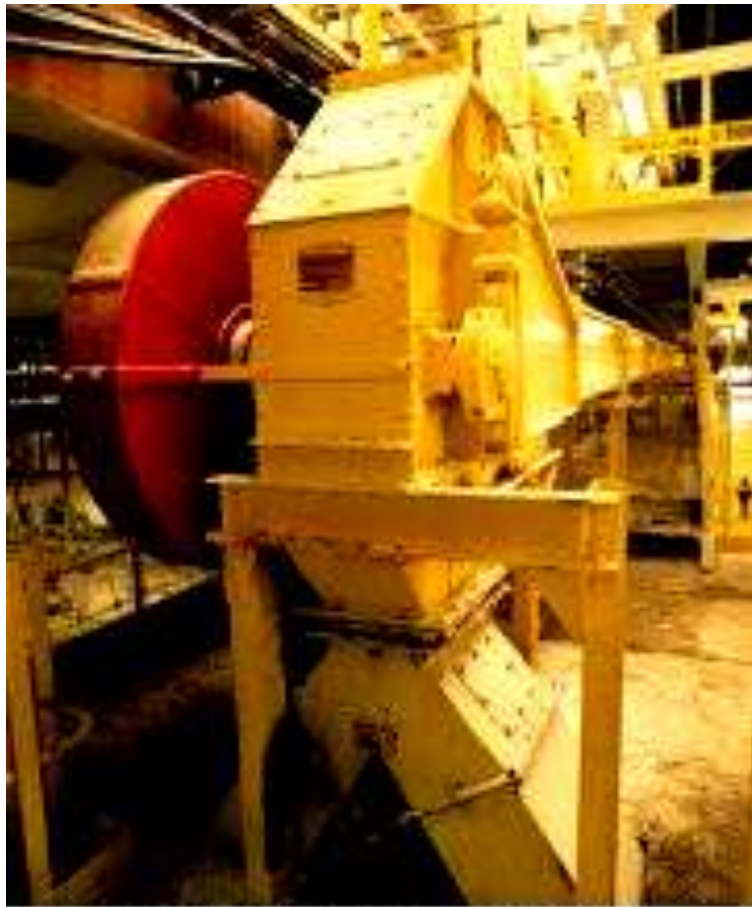
Conveying 50 tonnes per hour of soda ash at 150°C
