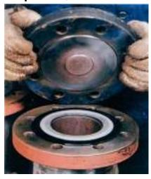
Gaskets are wound in V-section metal strip and a softer filler material. Support rings, inside and/or outside the spiral, improve the gasket's handling, fitting and versatility.
