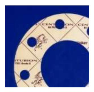
Centurion® is a high performance sheet jointing, based on glass and aramid fibres with a nitrile (NBR) binder. An anti-stick finish to both surfaces is supplied as standard.
