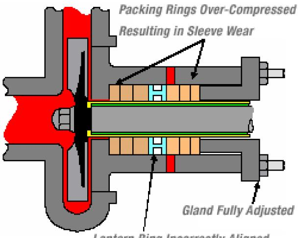
Lantern Ring Incorrectly Aligned, No Cooling Being Accomplished
